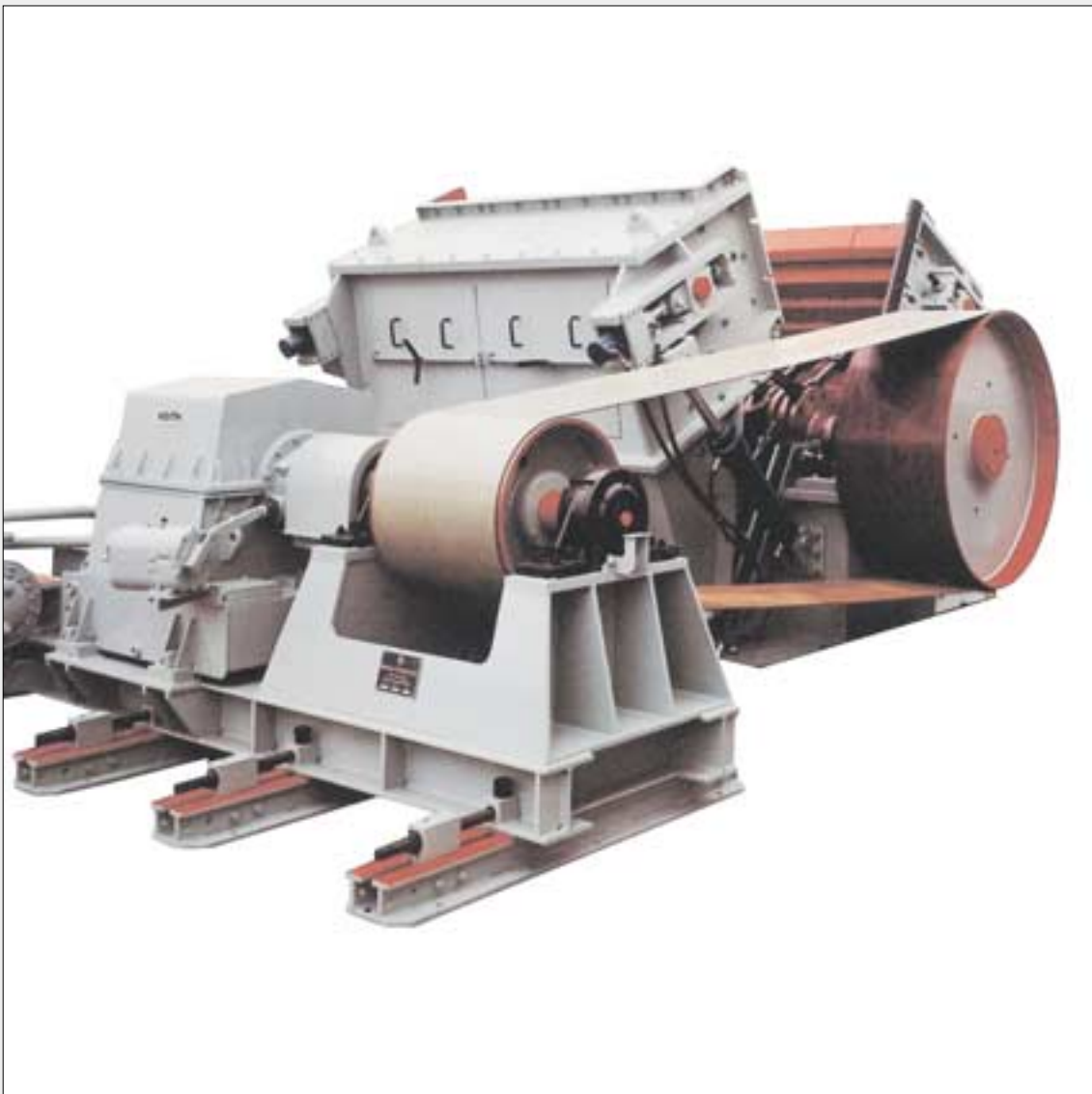
Prallspalter with regulating gear for the preparation of coking coal
