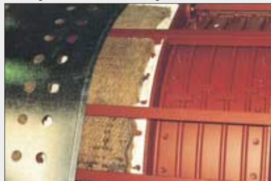
Heating with steam or heat-conducting oil
